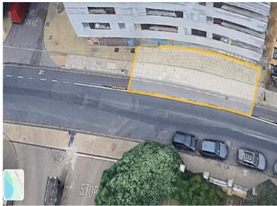
Block Nr.22 - Compound/Welfare Area (circa 28m x 6m) 2 x Containers @ 9.75m x 2.44m – double stack and 2 x Containers @ 7.35m x 2.44m – double stack
