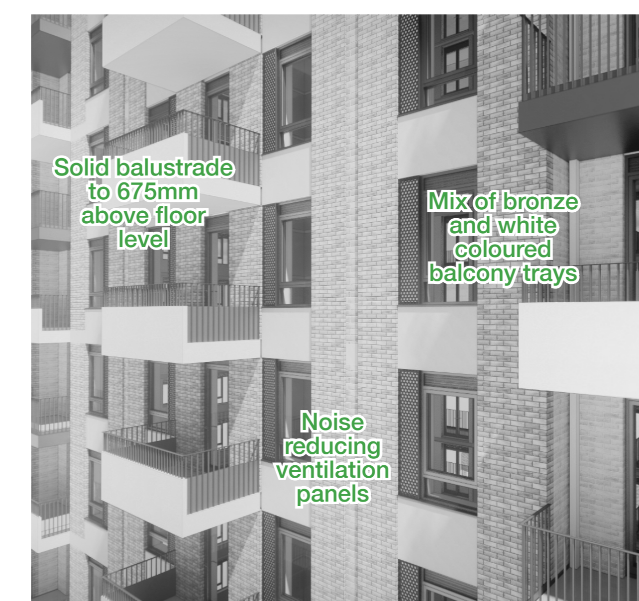
Balcony and vent detail
