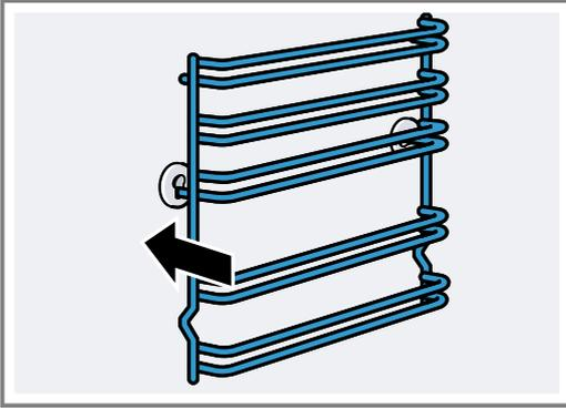
The rails fit both on the left and right sides. Shelf positions 1 and 2 are located at the bottom and shelf positions 3, 4 and 5 are located at the top.
