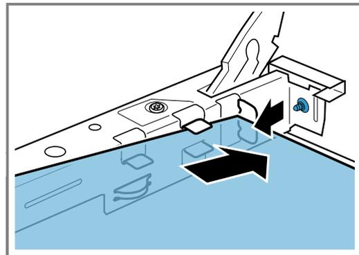
2. Hold the top pane in both brackets and insert it at an angle towards the back.
