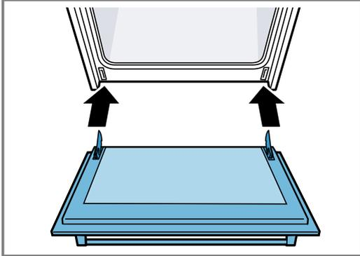
2. The notch on the hinge must engage on both sides.
