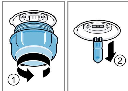
4. Insert the new halogen bulb and press it firmly into the socket.
